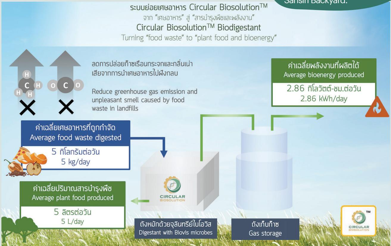
The process is done through fermentation buckets that transform food waste or organic waste into fertiliser and biogas, which can then be processed into high-capacity biomass for further generation into electricity.
